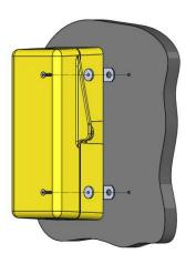
Wall mounting: Use reducing washers supplied with telephone Pole or post mounting: Stand-alone, battery powered with solar charger solution. Contact DAC for details.
