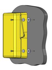
Wall mounting: Use reducing washers supplied with telephone Pole or post mounting: Stand-alone, battery powered with solar charger solution. Contact DAC for details. GSM/GSM-R Telephone PADS No. misc. Battery Pack PADS No. 087/038203
