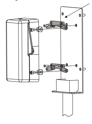
Ensure the top bracket is fixed using bottom holes and bottom bracket is fixed using top holes.
