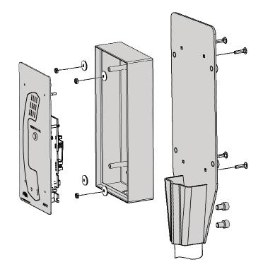
Wall mounting: On Wall box available from DAC: Part No. RA711-NR PADS No. 087/000666
